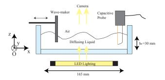
Figure 1. Experimental setup. A LED device ensures a homogeneous lighting below the transparent tank. A fast camera one meter above, is focused on the liquid free-surface. For comparison, the wave amplitude at some location is also recorded by a capacitive wave gauge.
