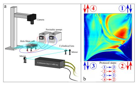
Figure 1. a: Sketch of the experimental setup. b: Time-periodic protocol and example of dye visualization.
