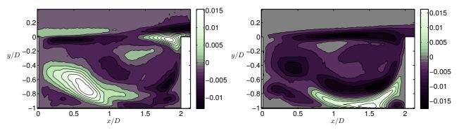
Figure 2. Example of global Fourier mode in a xy-plane, associated with frequency  $f D/U_0 = 0.024$ , for  $\text{Re}_D = 4570$ . Real part (*left*) and imaginary part (*right*) are depicted with contours of the streamwise velocity u', normalised by incoming velocity  $U_0$ .
