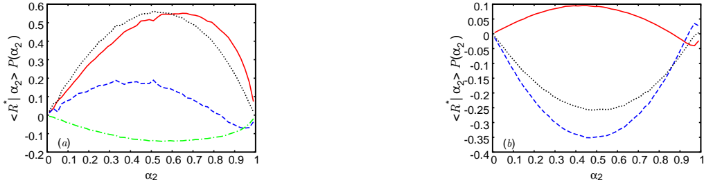
Figure 2. The probability fluxes \langle R^* | \alpha_2 \rangle P(\alpha_2) for \mathbf{e}_1^c - \mathbf{e}_2^s alignment at t = 3.68\tau_\eta . (a) Solid line: R_o^s ; dashed: R_p^s ; dash-dotted: R_v^s ; dotted: the sum. (b) Solid: R_o^c ; dashed: R_s^c ; dotted: the sum.
