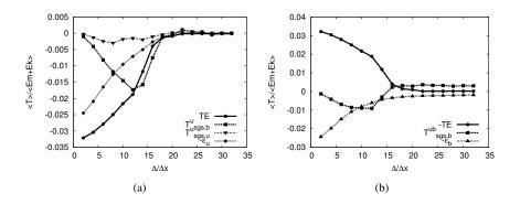
Figure 1. Energy transfers versus the filtering size  $\Delta/\Delta_x$  involved in (a) the kinetic energy equation (3), and (b) the magnetic energy equation (4), for a helical forcing.
