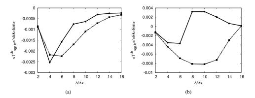
Figure 2. Energy transfer  $T_{sgs,b}^{ub}$  versus  $\Delta/\Delta x$  for (a) non-helical and (b) helical forcing. The solid line corresponds to the eddy magnetic diffusivity model [1] and the dotted line to the filtered DNS.
