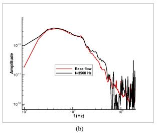
Figure 2. PSD of the base flow case and plasma controlled jet at  $f_p$ =3500 Hz, duty cycle 100%, for (a) the near field (x=2 Diameters) and (b) the far field (Polar angle =  $20^{\circ}$ ). Mach number : 0.3.
