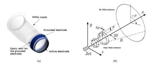
Figure 1. Sketch of the experimental setup: (a) nozzle and plasma actuator and (b) microphones distribution
