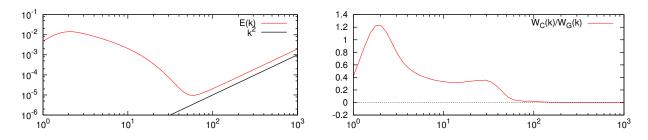
Figure 2. Left: Energy spectrum for truncated Euler flow. Right: spectrum of the nonlinear term, normalized by the Gaussian contribution.
