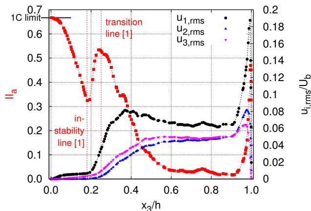
Figure 2: Development of the second anisotropy invariant,  $\Pi_a$ , and the normalized rms-values of the velocity fluctuations,  $u_{i,rms}$ , along the  $x_3$ -axis (note: irregularities in the data result from the nature of the unstructured grid and the presently limited spatial interpolation of the data).
