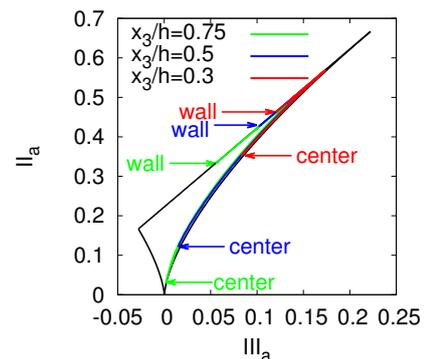
Figure 3: Trajectories in the anisotropy invariant map at three spanwise positions in the triangular duct.
