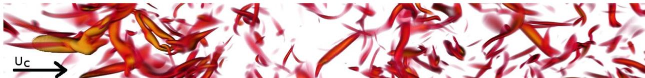
**Figure 1.** Turbulent wake of a particle located at the left side of the simulation box at  $Re_p = 400$  (defined with the mean flow  $U_c$ ). The advected flow is turbulent with  $I = 0.14$  (volume rendering of high-vorticity isosurfaces).
