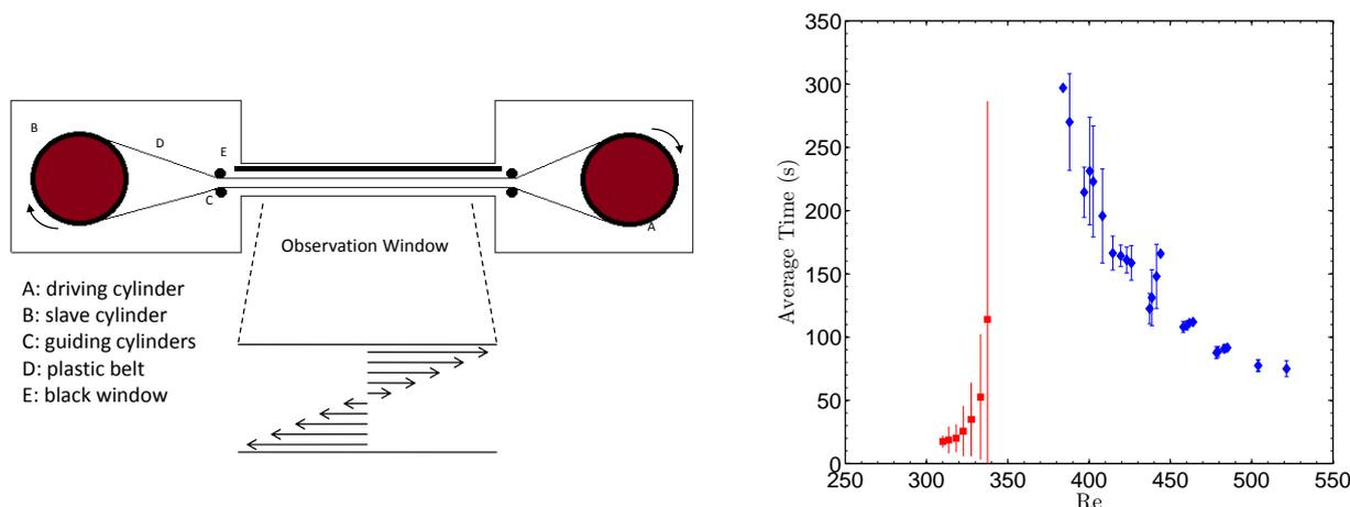
**Figure 1.** Left: sketch of the experimental setup. Right: averaged time to observe a fully turbulent or fully laminar flow during a cold start or a quench experiment respectively as a function of the final  $Re$ . See text for details.
