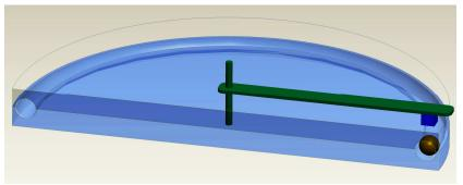
Figure 1. Sketch of the experimental setup used to realize a constant flow rate in a torus: two disks of perspex into each of which a concentric notch of half-circular cross sections has been machined, and a rotating boom driving a sphere by means of a magnet. The sphere hence drives the flow.
