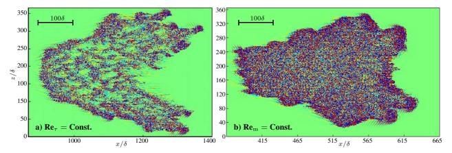
Figure 1. Contours of instantaneous wall-normal velocity in the channel central plane, showing the spot shape and inside structures during the spot evolving at  $tu_{\tau 0}/\nu = 3360$  for the constant driving force (a) and at 1790 for the constant mass flux (b). Red and blue colors indicate positive and negative values, respectively, while green represents zero. The mean flow direction is from left to right. The horizontal axis denotes the distance from the trigger point of the spot.
