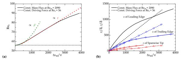
Figure 2. Temporal variations of friction Reynolds number (a) and positions of stream- and spanwise edges of spot (b).
