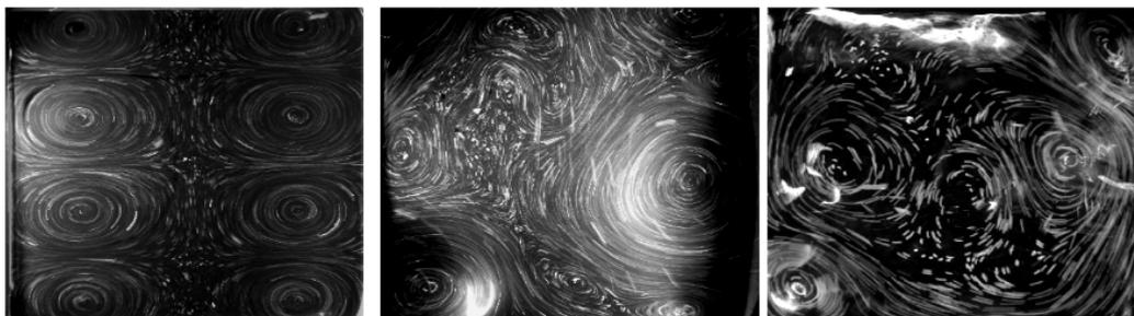
**Figure 1.** Photographs of the three different regimes, from left to right: laminar regime (with the 8 counter-rotating vortices), turbulent regime and condensate state.
