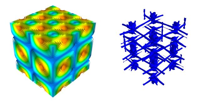
Figure 1. Isosurfaces of velocity magnitude for vortex array,  $u = \cos x \sin x \cos z$ ,  $v = -\sin x \cos y \cos z$ , w = 0 on  $(0, 2\pi) \times (0, 2\pi) \times (0, 2\pi)$ , (left), and  $\lambda_2 = -0.15(\lambda_2)_{\text{max}}$  iso-surface (right). The flow is periodic with a period of  $2\pi$  in each direction.
