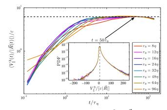
**Figure 2.** Time evolution of the average local rate of kinetic energy transfer  $\langle V_{\parallel}^3(t)/|\vec{R}(t)|\rangle$  for various initial separations between the particles. Inset: Probability density function of  $V_{\parallel}^3(t)/|\vec{R}(t)|$  at time  $t = 50\tau_{\eta}$  and for the same initial separations.
