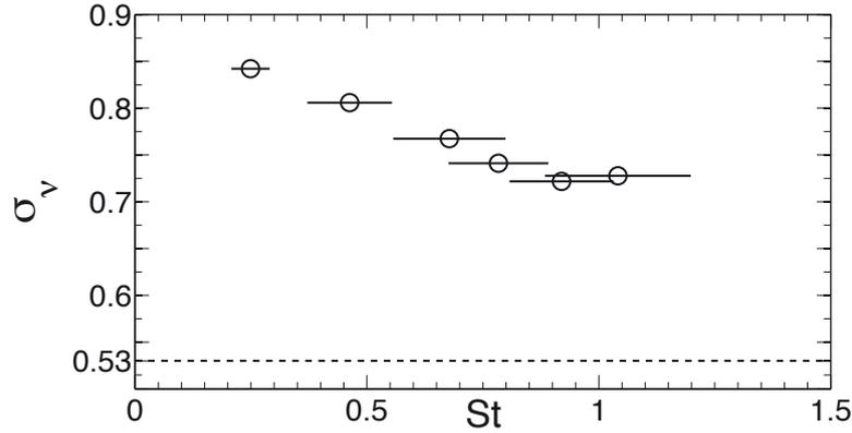
**Figure 2.** Preliminary result: evolution of the clustering diagnosis (namely the standard deviation  $\sigma_V$  of the normalized Voronoï areas) with entangled Stokes and Reynolds numbers. The dashed line is the standard deviation of a Random Poisson Process (*i.e.* a seeding with no spatial structuring), of value  $\sigma_{RPP} \approx 0.53$ .
