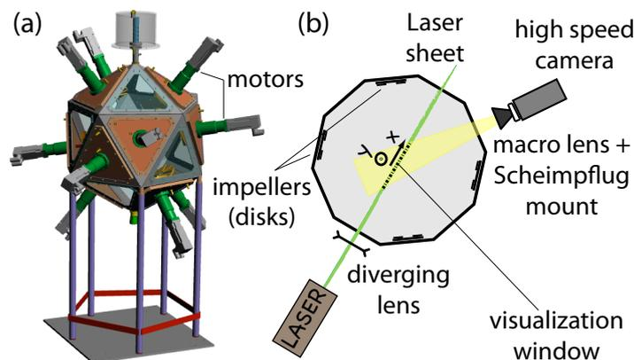
**Figure 1.** (a) CAD drawing of the LEM. (b) Schematic upper view of the setup.
