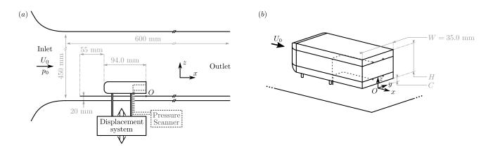
Figure 1. (a) Experimental set-up of the model in the wind tunnel; O sets the origin of the coordinate system. (b) Scheme of the body; grey dots on the base are pressure taps; for clarity, only the pressure tubings from the two taps in the field y < 0 are displayed.
