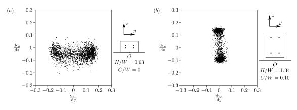
Figure 3. Instantaneous pressure gradients in the y and z directions: (a), H/W = 0.63 and C/W = 0; (b), H/W = 1.34 and C/W = 0.10.
