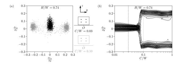
Figure 2. (a) Instantaneous pressure gradients in the y and z directions for H/W = 0.74: C/W = 0.03 (black dots) and C/W = 0.10 (gray dots). (b) Probability density function of the base pressure gradient in the y direction as a function of the ground clearance for H/W = 0.74; contour intervals are 1.
