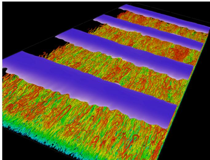
**Figure 4.** Visualisation of the turbulence on the unstable (bottom) side and a developing instability on the stable (top) side of a channel flow at  $Re_b = 20000$  and  $Ro_b = 1.2$ .
