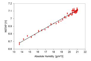
Figure 2. Preliminary results indicating the sensitivity to humidity of the new fast-response humidity sensor.
