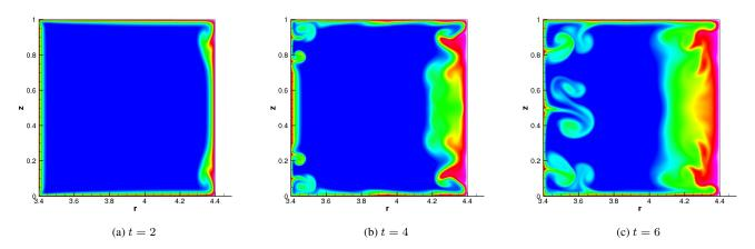
Figure 2: Contour plots of the azimuthal velocity component w in the case of a toroidal container spun up from rest. Show are three time snaps taken at (a) t = 2, (b) t = 4 and (c) t = 6 for a flow with a Reynolds number Re = 2000.
