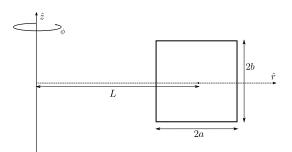
Figure 1: A cross-section of the annulus, with dimensional centreline radius L and cross-sectional radii a and b, in the rand z-directions respectively. The outer wall of the annulus is at  $\hat{r} = L + a$ , whilst the inner wall is at  $\hat{r} = L - a$ . The upper wall of the annulus is at  $\hat{z} = b$ , with the lower wall is at  $\hat{z} = -b$ .
