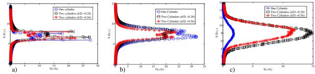
Figure 3. Turbulence intensity profile. a) Station X/D = 0.1, b) Station X/D = 4, c) Station X/D = 20.
