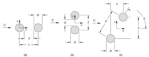
**Figure 1.** Two circular cylinders of equal diameter in cross-flow: (a) tandem configuration; (b) side-by-side configuration; and (c) staggered configuration.
