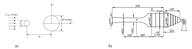
Figure 2. Schematic of a) passive flow Over the rod and Circular Cylinder, b) wind tunnel dimension.
