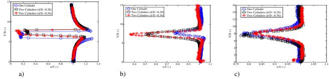
Figure 4. Velocity profile. a) Station X/D = 0.1, b) Station X/D = 4, c) Station X/D = 20.
