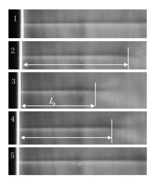
Figure 1. Schlieren-visualization of the flow field of microjet outflowing from the nozzle diameter of 35 microns.
