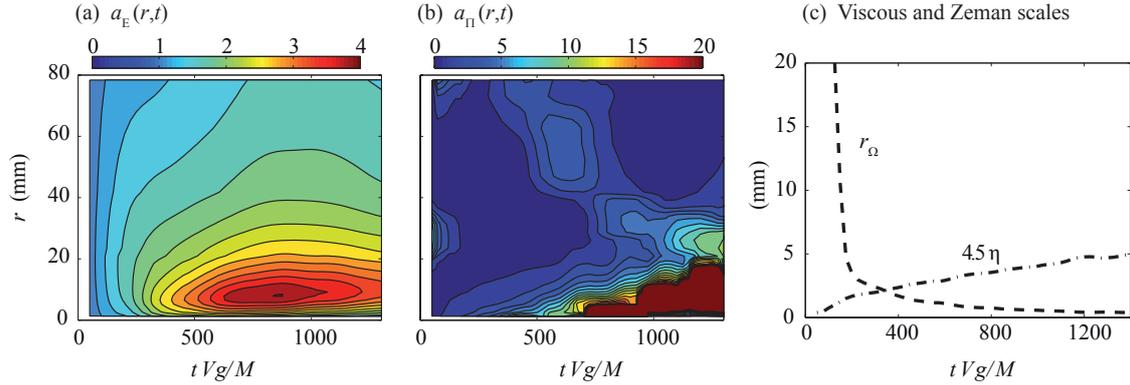
**Figure 1.** (a,b) Spatio-temporal diagrams showing the ratio of the horizontal-to-vertical energy  $E$  (a) and energy flux  $\Pi$  (b) in a decaying turbulence rotating at  $\Omega = 16$  rpm. (c) Time evolution of the Zeman scale  $r_\Omega$  and of  $r_\nu = 4.5\eta$  which measures the cutoff scale between the transfer and viscous terms of the KHM equation (3) ( $\eta$  is the Kolmogorov scale).
