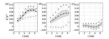
Figure 2. Evolution of magnetic profile with N. (a) Hydrodynamic regime  $N \ll 1$ . (b) Transition regime  $N \sim 0.1$ . (c) MHD regime  $N \sim 1$ . Blacks curves represents mean profiles and other curves represents the furthest profile from the mean. Grey area shows the rms of the profiles.
