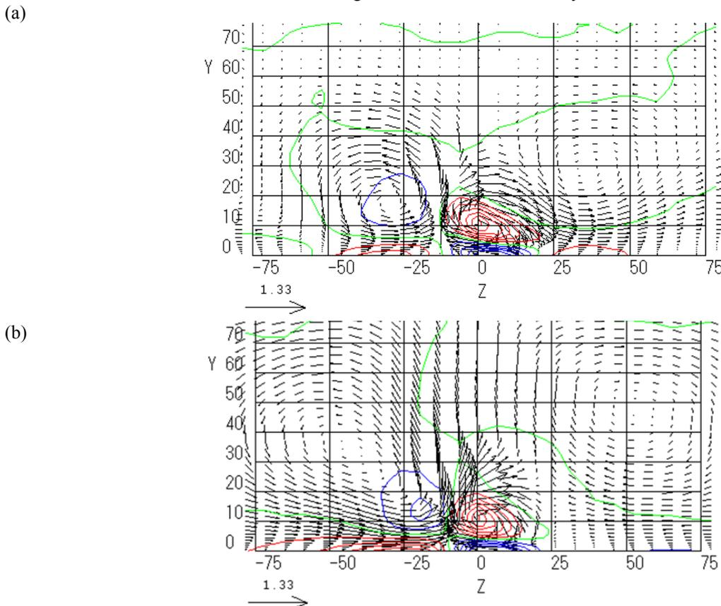
**Figure 2.** Averaged velocity vectors  $v$  and  $w$  and contours of streamwise vorticity in the cross streamwise plane; Red and blue contours represent positive and negative vorticity, while green represents zero vorticity. All quantities are non-dimensionalized by mean pressure gradient, channel half width and viscosity.  $Y$  and  $Z$  are non-dimensionalized by the viscosity and friction velocity. (a)  $Ro=0.25$ , (b)  $Ro=1.5$ .
