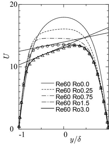
**Figure 1.** Mean velocity profiles. Mean velocity is normalized by the mean pressure gradient and channel half width. Symbols represent the numerical simulations of 512 x 129 x 288 grid points. Tangent lines are included to show the region of zero absolute vorticity.
