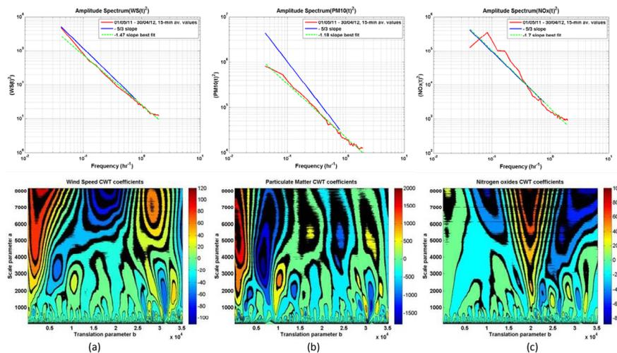
**Figure 1.** Air quality and meteorological timeseries data analysis. (a) Wind Speed (b) Particulate Matter of size at least  $10\mu m$  (c) Nitrogen Oxides the timeseries plot (top); the spectral energy distribution (middle), and CWT analysis (bottom) for each variable
