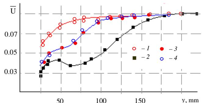
**Figure 2.** Velocity scaled on ship model velocity around the propeller disc: 1 – smooth surface, WSR-301 solution, concentration  $\sim 6 \cdot 10^{-4} \%$ ; 2 – rough surface, water; 3 – rough surface, WSR-301 solution, concentration  $\sim 4.5 \cdot 10^{-4} \%$ ; 4 – smooth surface, water.
