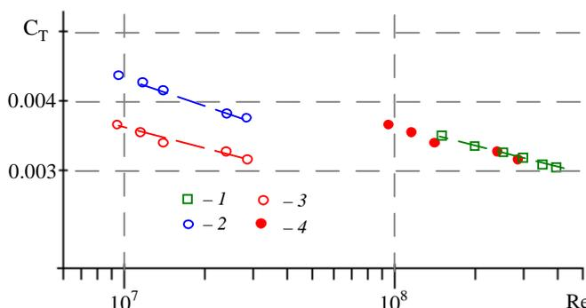
**Figure 1.** Dependence of total resistance coefficient on  $Re$ : 1 – sea trials, underwater vehicle; 2 – towing tank, UV model; 3 – towing tank, UV model, polymer drag reduction  $\sim 30\%$ ; 4 – shift in  $Re$  on the order of magnitude for the case 3.
