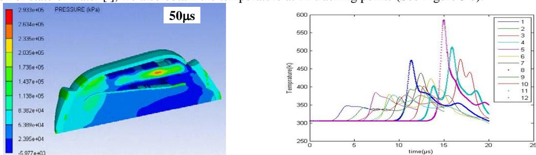
**Figure 5** Pressure field in the container and the temperature at 12 tracking points
