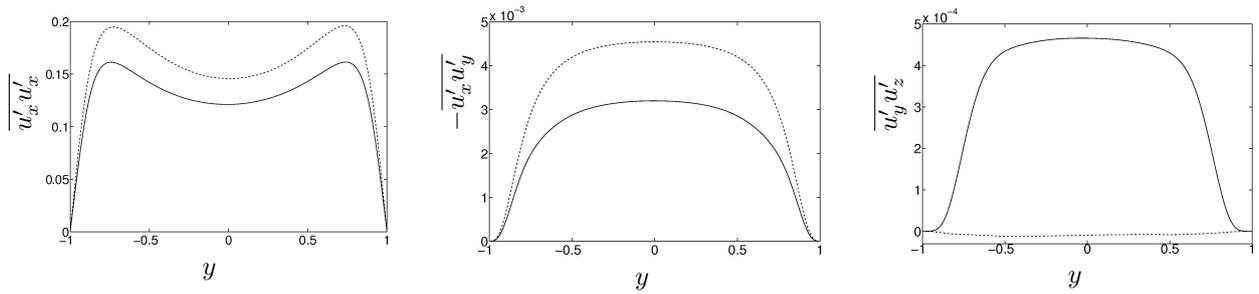
**Figure 2.** Reynolds stress tensor components for unmanipulated turbulent (---) and controlled (—) flows.
