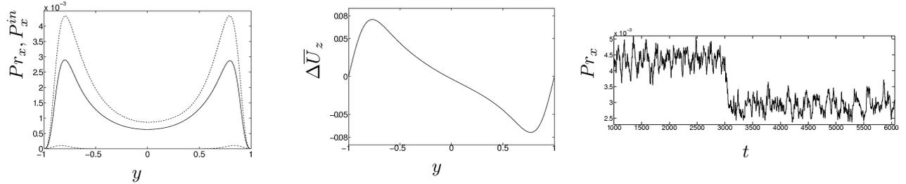
**Figure 3.** Left plot: Time averaged productions of turbulent kinetic energy ( $Pr_x$ ) for the turbulent (---) and controlled (—) flows and input power,  $P_x^{in}$ , (— · —); Middle plot: The deviation of the controlled flow mean spanwise ( $\Delta \bar{U}_z$ ) velocity profiles from the unmanipulated turbulent flow ones; Right plot: Time evolution of  $Pr_x$  for the unmanipulated ( $t < 3000$ ) and controlled ( $t > 3000$ ) flows (right plot).
