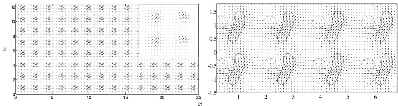
**Figure 1.** Left plot: the design of the helical forcing in  $xz$ -plane at  $y = -0.95$ ; Right plot: the related seed velocity field imposed at each action of the forcing in the same plane with contours of positive (0.0005 —) and negative (−0.0001 - - -) spanwise velocity.
