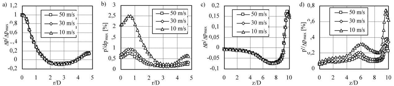
**Figure 3.** Radial and axial redistribution of static pressure and its fluctuation for distains between outlet of pipe and impinging jet 10D: a, b – impinging wall; c, d – side wall
