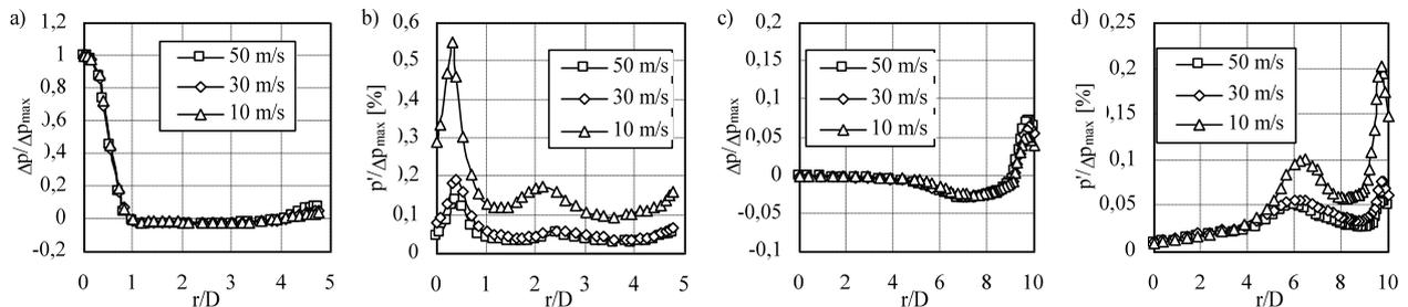
**Figure 4.** Radial and axial redistribution of static pressure and its fluctuation for distains between outlet of pipe and impinging jet 1D: a, b – impinging wall; c, d – side wall
