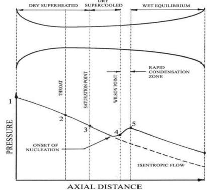
Figure 1. Variation of axial pressure for the steam expansion on the Laval nozzle centerline
