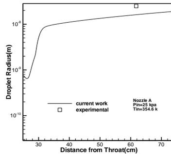
Figure 3. Theoretical and experimental data of droplet radius in center line of nozzle.
