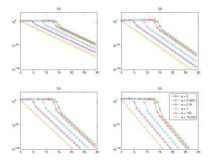
Figure 1. Semi-log plot of compensated structure functions,  $S_n(k) \cdot k^{n/3}$ . Viscosity =  $\nu = 10^{-12}$  and several values of  $\alpha$ .
