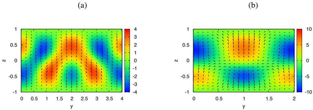
**Figure 2.** The cross-sectional velocity structure at  $x = (1/4)(2\pi/\alpha)$ .  $R = 100$ . The colour code indicates the streamwise velocity component. (a):  $\mathcal{A}_0$  (or *Ribbon*) with  $(\alpha, \beta) = (0.8, 1.56)$  at  $\Omega = 13$ . (b):  $\mathcal{A}_3$  with  $(\alpha, \beta) = (1.6, 3.12)$  at  $\Omega = 20$ .
