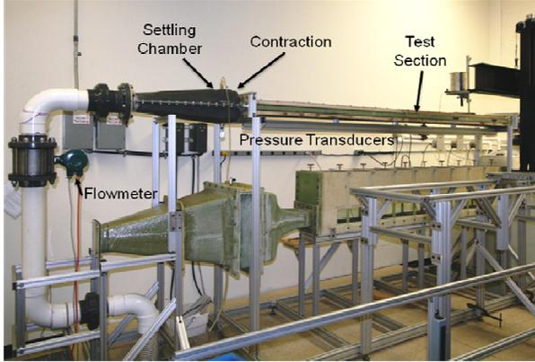
Figure 1. Fully developed channel flow facility.
