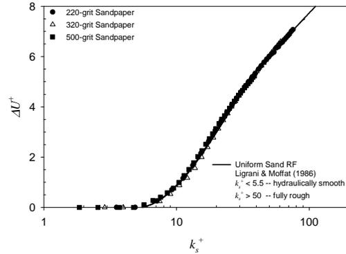
Figure 4. Roughness functions for sandpaper roughness.
