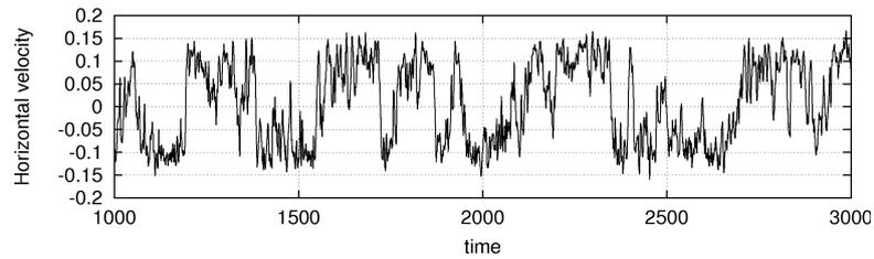
**Figure 1.** Time series of horizontal velocity in the bottom boundary layer. Time units are given in dimensionless form, calculated from the natural convection velocity as the reference velocity.
