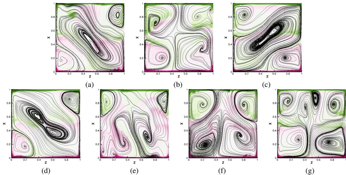
**Figure 2.** Snapshots of the streamlines on the vertical midplane colored by the temperature.
