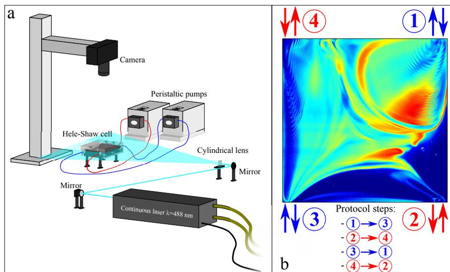
**Figure 1.** a: Sketch of the experimental setup. b: Time-periodic protocol and example of dye visualization.
