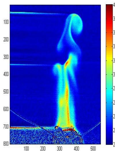
**Figure 1:** Temperature field around a plume emitted from a small heating element. The temperature scale is on the right in celcius.
