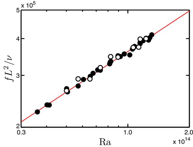
**Figure 2.** The non-dimensional frequency  $\tilde{f} = fL^2/\nu$  associated with the LSC versus the Rayleigh number. Closed circles: the frequency  $\tilde{f}_C$  as obtained from the cross-correlation function  $C_{t,m}^{b,m}$ . Open circles: the frequency  $\tilde{f}_L$  as obtained from the single-point frequency power spectrum  $P(f)$ . A power-law fit to the cross-correlation data results in  $\tilde{f}_C \propto Ra^{0.46}$  as indicated by the solid red line.
