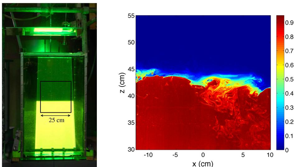
**Figure 1.** Left: experimental setup. Right: snapshot of the density field (red, close to one: dense fluid; blue, close to zero: light fluid) in the 25cm×25cm area.
