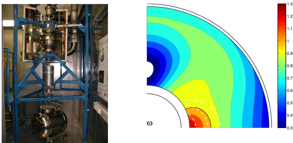
**Figure 1.** The picture on the left hand side is the DTS setup in Isterre sodium lab (Grenoble). On the right hand side we plotted the meridional Angular velocity mean flow in the sodium shell. Solution is abtained from experimental data inversion. Velocity is normalized to the inner sphere rotation frequency.
