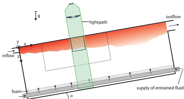
Figure 1: Sketch of the experimental facility including PIV measurement setup
