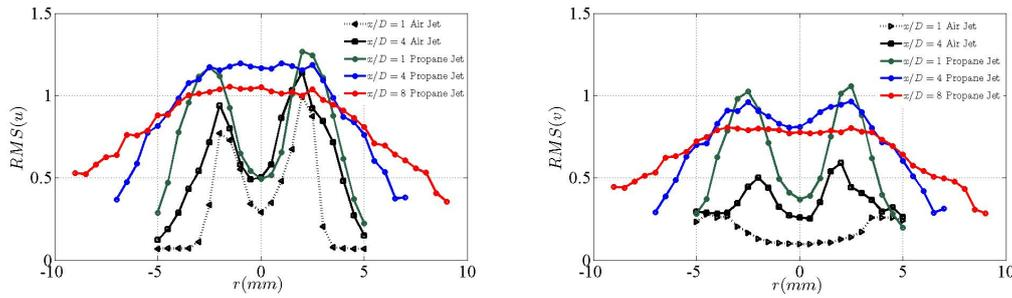
**Figure 2.** Standard deviation of fluctuating velocity profiles  $\overline{u'^2}^{1/2}$  (left) and  $\overline{v'^2}^{1/2}$  (right) for propane (VVF) and air (CVF) jets.  $M_0=130 \text{ kg/m}^2/\text{s}^2$ , for  $x/D=1, 4$  and  $8$ .
