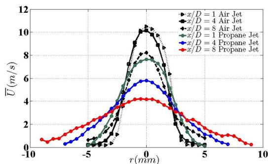
Figure 1. Radial mean velocity profiles  $\bar{U}(r)$  for air (left) and propane (right) jets at  $M_0=130 \text{ kg/m}^2\text{s}^2$ , as a function of the radial position  $r$  normalised with respect to the jet half-width  $y_{1/2}$ , at three downstream positions  $x/D = 1, 4$  and  $8$ .
