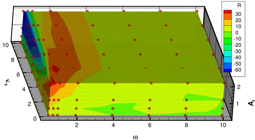
**Figure 1.** The map of drag reduction in parametric space  $\omega - \kappa_z - A$  at  $\Delta = 0.01$ . Each red dots on the map correspond to a DNS simulation. The contour of  $R(\%)$  is drawn based on linear interpolation.  $R > 0$  indicates drag reduction while  $R < 0$  indicates drag increase cases.
