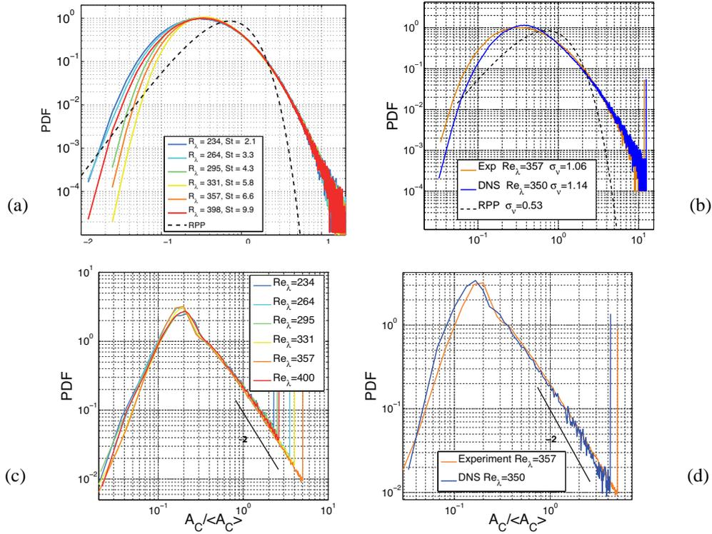
**Figure 1.** (a) Probability distribution of normalized Voronoi area  $\nu$  for different Reynolds and Stokes numbers. (b) PDF of normalized Voronoi area  $\nu$  for the experiment (orange line) and the simulation (blue) for  $Re_\lambda$  350. In both figures the black dashed line is a RPP distribution. (c) PDF of normalized clusters area for experiments. (d) PDF of clusters area for the experiment (orange line) and the simulation for  $Re_\lambda$  350 (blue)
