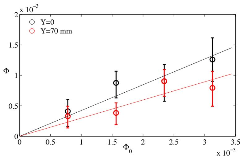
**Figure 1.** Relationship between local volume fraction  $\Phi$  and the volume fraction averaged over the entire stirred tank  $\Phi_0$ . Comparison of the two shows the effect of gravitational settling.
