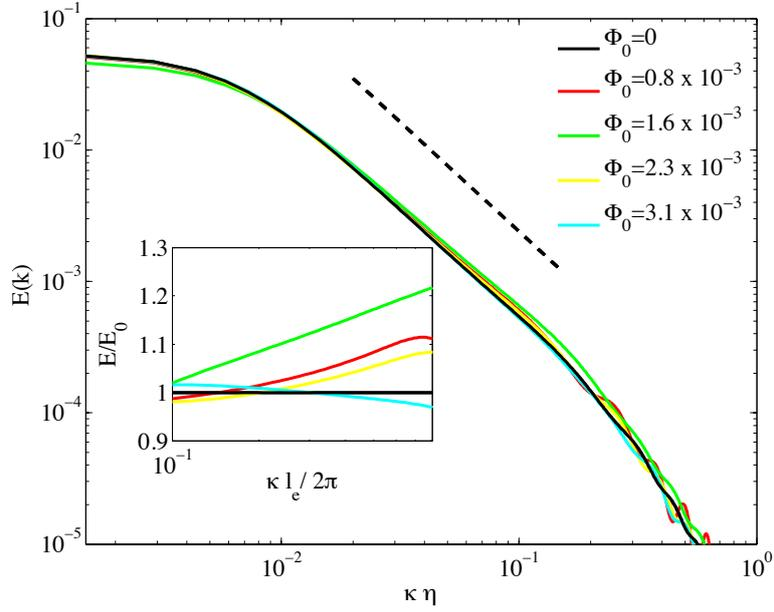
**Figure 2.** Power spectrum for increasing particle concentration showing spectral tilting (Black:  $\Phi_0 = 0$ , Red:  $\Phi_0 = 0.8 \times 10^{-3}$ , Green:  $\Phi_0 = 1.6 \times 10^{-3}$ , Yellow:  $\Phi_0 = 2.3 \times 10^{-3}$ , Cyan:  $\Phi_0 = 3.1 \times 10^{-3}$ ). The inset shows the relative change of the spectra (compared to single-phase) on a scale relative to the particle size  $l_e$ . The blue line shows the 'reverse pivot'.
