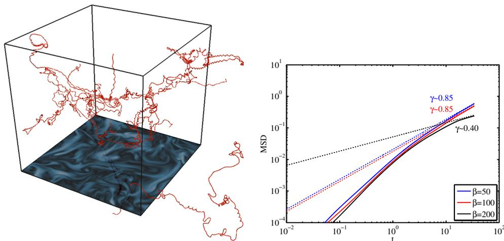
**Figure 1.** Left: sample charged particle trajectories in an MHD field obtained from Direct Numerical Simulation (resolution:  $512^3$  modes,  $Re_\lambda \approx 250$ ). The bottom cut represents the local intensity of the magnetic field. Right: average square mean displacement of a sample of  $5 \times 10^5$  particles for different values of the coupling parameter  $\beta$  (the symbol  $\gamma$  represents the slope of the curves for large times) [4].
