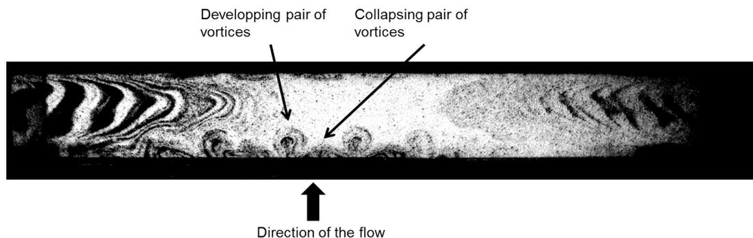
**Figure 1.** Top view of the cavity : smoke visualization of the secondary phenomenon.
