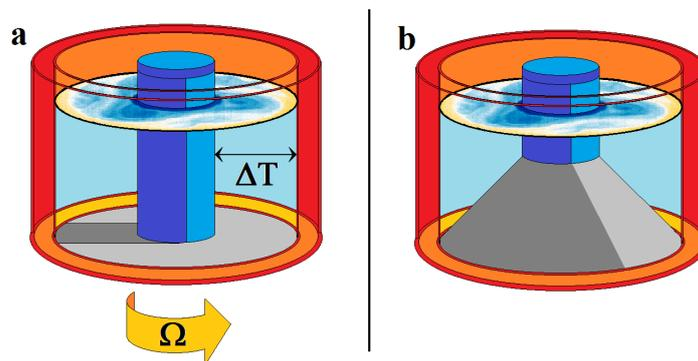
**Figure 1.** The schematic drawing of the geometry of our experimental setup in the flat bottom case (a) and with sloping bottom topography (b).
