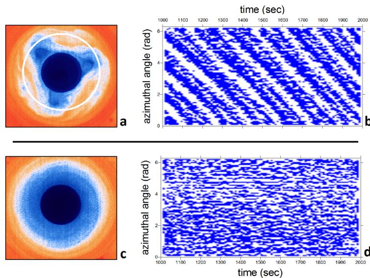
**Figure 2.** A thermal snapshot (a) and the propagation (Hovmöller) plot (b) of a stable regular wave at  $Ta = 5.78 \cdot 10^6$ ,  $Ro_T = 1.56$ , and of a typical axisymmetric experimental run at  $Ta = 3.57 \cdot 10^6$ ,  $Ro_T = 2.55$  (c and d). The propagation plots depict the temporal development of temperature anomalies taken along the path marked by a white circle in (a). The white data points indicate warmer-than-average, while the blue depict colder-than-average temperature.
