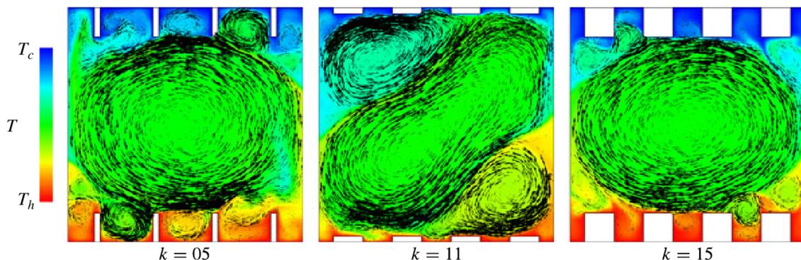
**Figure 1.** Instantaneous temperature field in two-dimensional DNS for different configurations ( $k$ ) of roughness,  $Ra = 10^8$ ,  $Pr = 1$  (adopted from [7]).
