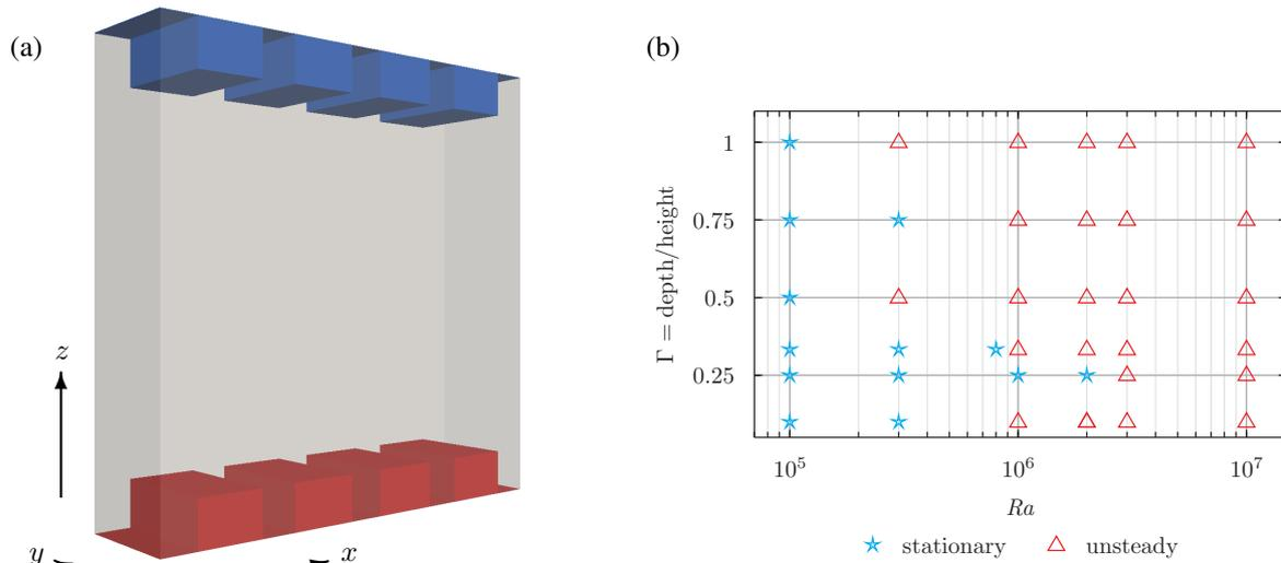
**Figure 2.** (a) Sketch of the considered quasi two-dimensional geometry for investigating the influence of roughness. The quantity of the heated/cooled obstacles on the bottom/top plate and their size may vary. (b) Influence of the aspect ratio  $\Gamma = \text{depth/height}$  on the state of the equilibrium for smooth no-slip walls,  $Pr = 0.786$ .
