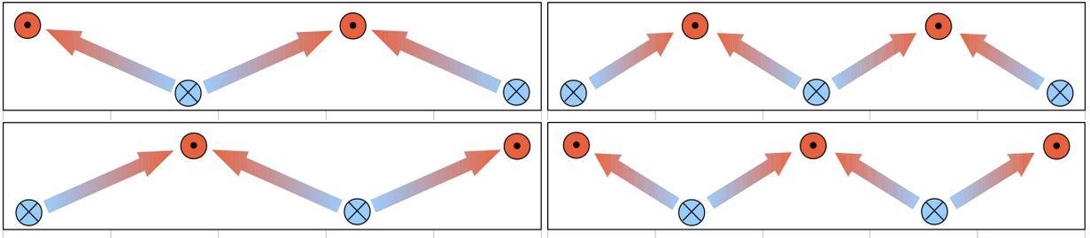
**Figure 3.** View from above on a layer close above the bottom plate, e.g. the layer with the temperature probes sketched in Fig. 1. Arrows indicate the direction of the in plane movement,  $\odot$  up- and  $\otimes$  downstreaming fluid and the colour scales with the temperature. Top left: three LSCs, top right: four LSCs, bottom left: three LSCs counter rotating and bottom right: four LSCs counter rotating.
