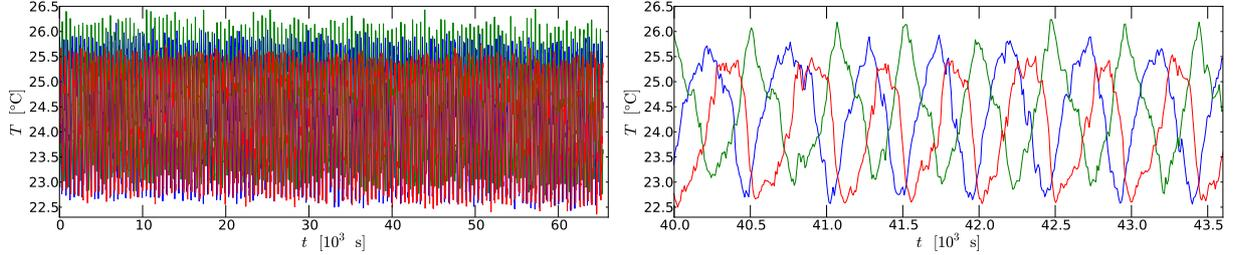
**Figure 2.** Temperature time series recorded at three selected sensor positions: P1 —, P2 — and P3 — at a parameter combination with periodically oscillating LSCs. Left: total recorded measurement time, right: detailed view of one hour.
