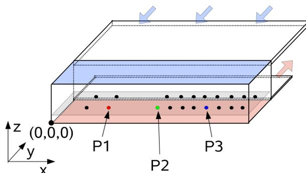
**Figure 1.** Sketch of the convection cell. The bottom plate of the cell is heated (red) while the ceiling is kept at the ambient temperature (blue). The in- and outflow channels are located at the same side wall and span the whole length of the cell. Dots mark the positions of the PT-100 sensors in the layer  $Z/H = 0.2$  within the cell. More PT-100 sensors are placed in the layer  $Z/H = 0.8$ , but are not shown for the sake of clarity.
